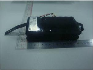
Cell/电芯 (Panasonic#NCR18650A 3,6V 2900mAh)
