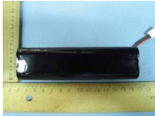
电池/Battery (24-530001-03 7,2V 5900mAh 42,48Wh)
