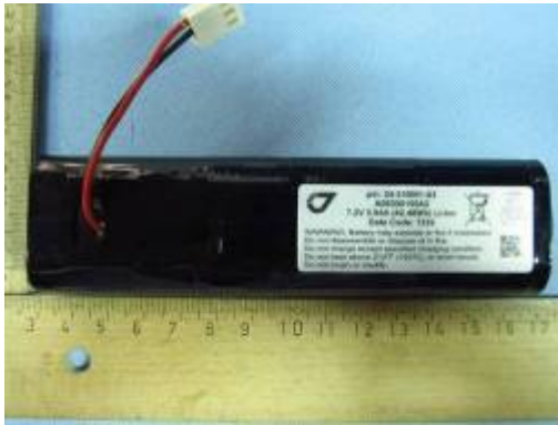
电池/Battery (24-530001-03 7,2V 5900mAh 42,48Wh)
