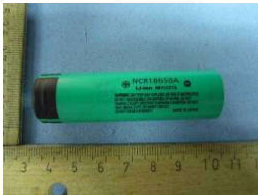
电芯/cell(NCR-18650A 3,6V 2950mAh 10,6Wh)
