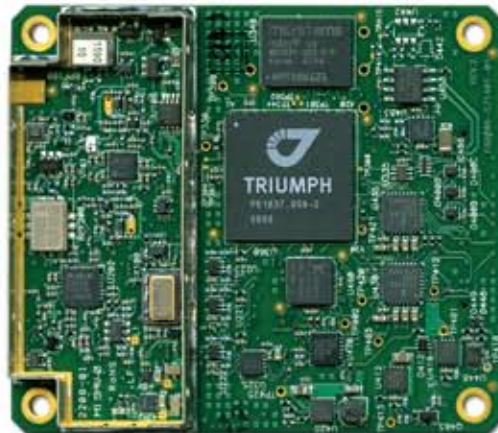
TR-G2T 16 EACH OF GPS L1/L2/L2C/L5, GALILEO E1/E5A
