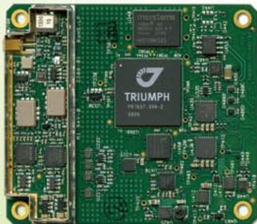
TR-G3 16 EACH OF GPS L1, GALILEO E1, GLONASS L1
