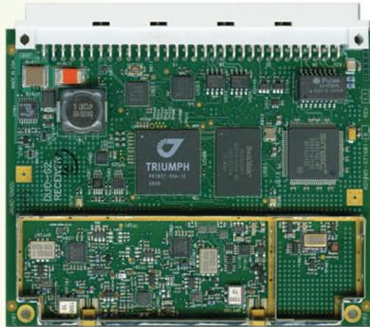
DUO-G2 TWO SETS OF 14 EACH OF GPS L1, GALILEO E1
