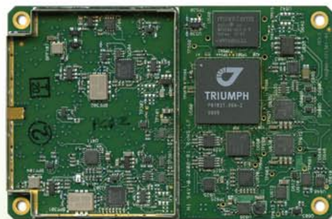
TR-G3T 16 EACH OF GPS L1/L2/L2C/L5, GALILEO E1/E5A, GLONASS L1/L2
