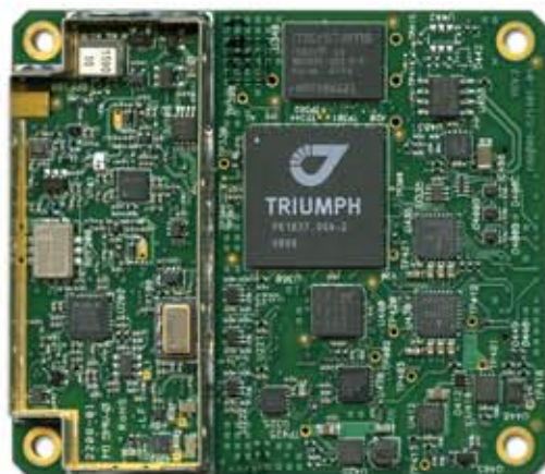
TR-G2T 16 EACH OF GPS L1/L2/L2C/L5, GALILEO E1/E5A
