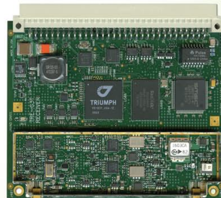
TRE-G3T 16 EACH OF GPS L1/L2/L2C/L5, GALILEO E1/E5A, GLONASS L1/L2 TRE-G3T-AJ HAS THE ANTI JAMMING CAPABILITY
