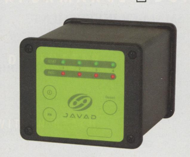
JNSGyro-2 is a dual frequency satellite-based two-antenna system that measures true heading. It contains two 20-channel geodetic quality dual frequency GPS (GLONASS optional) receivers packaged in one small box (159 x 49 x 138 mm) that is connected to two antennas whose base-line is fixed at the time of installation. The JNSGyro-2 can also be operated in RTK or DGPS mode from an external base station to provide highly accurate position and velocity.
