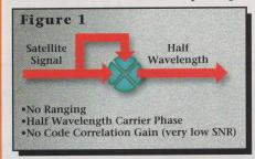
rules out the use of the 86cm L2 - L1 widelane observable since it halves the L2 carrier wavelength.
