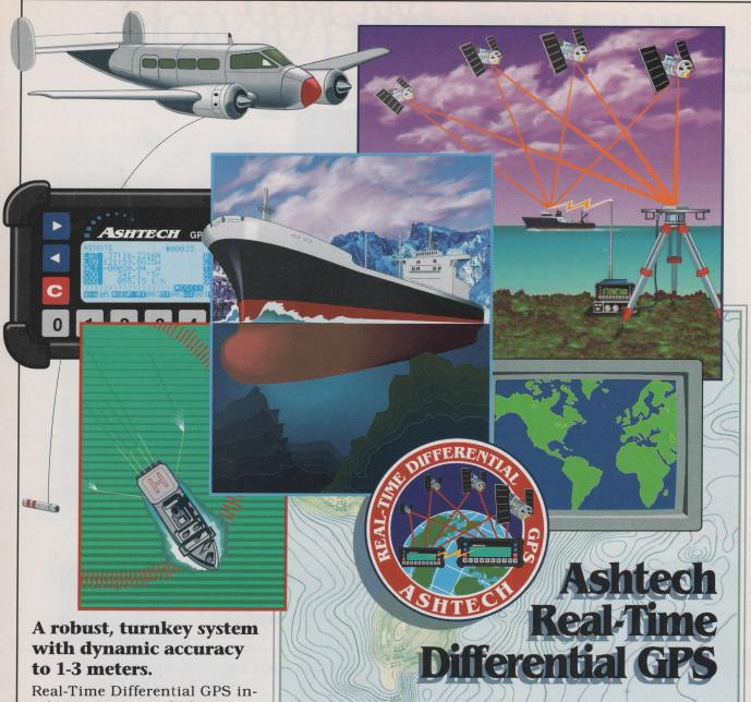
Real-Time Differential GPS involves operating a GPS receiver (Base) at a known location, where it observes the range errors of each GPS satellite and broadcasts corrections directly to a mobile GPS receiver (Remote) by radio, phone or other communications link. The remote's software then makes an integrity assessment and computes an instantaneous position fix.
