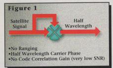
rules out the use of the 86cm L2 - L1 widelane observable since it halves the L2 carrier wavelength.
