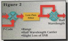
underlying P-Code, narrowing the bandwidth and subsequently squaring. This results in a half-wavelength carrier-phase observable and a signal-to-noise 17dB lower than that obtained by correlating with the P-Code.
