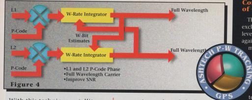
With this technique, satellite signals are correlated with locally generated versions of the P-Code (no cross-correlation) and integrated over W-Code chip intervals.
