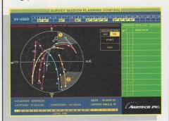
Mouse-driven graphics add new dimensions to GPS survey planning and post processing. Satellite SkyPlot shows elevation and azimuth as well as site obstructions; Visibility Chart identifies local rise and set times.
