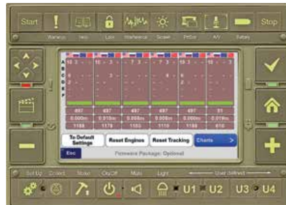
Six parallel RTK engines.
