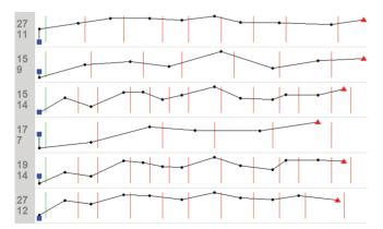
Expanded view of the vertical solution of each engine. Vertical red lines show the instants in which each engine has been reset and ambiguity solutions recalculated.
