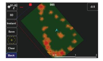
2D view of the field shows the magnetic objects that have been scanned.
