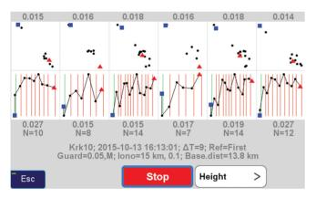
Phase-1 horizontal and vertical solution of each engine for each epoch.
