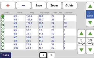
The top two graphs show the 3D view of the magnetic objects in the field. The following four screens show the digitized version of the 2D view. The mag data collected can be saved and recalled for further viewing and documentation. The "List" button lists the magnetic objects detected and their characteristics. Zoom button shows details of the selected object. Guide button will guide to the selected item.
