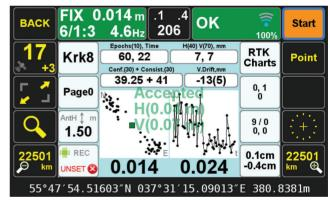
We have not only integrated a sophisticated magnetic locator in the TRIUMPH-LS, but we have also streamlined the whole process. First, the "Stakeout" screen will guide you towards the target.
