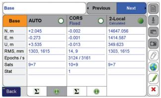
Initial base position can also be corrected by the rover occupying one or more known positions. This screen shows the initial and corrected positions of the base both by CORS and by m-Local known rover occupations.
