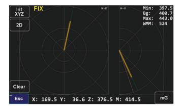
Horizontal and vertical magnetic vectors show the instantaneous vectors from the current position to the mag point.
