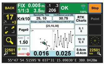
This graph shows the horizontal and vertical RTK epochs of Phase-1 along with their statistics. Each epoch is the average of six RTK engines.
