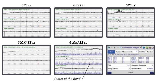
TRIUMPH-VS not only scans the GNSS bands and shows the shape and frequencies of the interferences, but it also quantifies the magnitude of the interferences in two distinct and complementary ways: a) by analyzing the analog signal and determining the "Interference Magnitude", and b) by analyzing the S/N (Signal-to-Noise ratio) of all satellites' signals after they are digitized and processed (after code and carrier correlations) and determining the "Satellites S/N loss" due to interferences.
