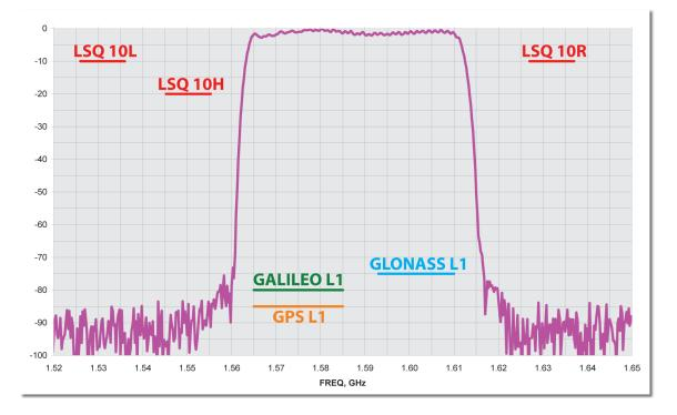
A good GNSS receiver should bring in ALL of wideband GNSS signals and reject all other unwanted signals. We announced the existence of this technology months ago for the L1 band. Now we have improved this filter and added similar protection for all other GNSS bands.
