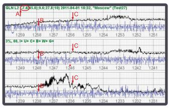
We have assigned 60 of our 216 GNSS channels to monitor the 6 GNSS bands and report interferences in four different ways. You can check interferences in your environment before starting your job to ensure your environment is clean.
