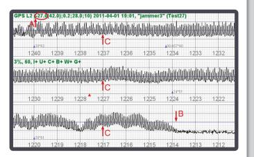
This figure shows color coded satellite signal strength after signal processing. Blue: Perfect, green: 3dB less, red: at least 6 dB less.
