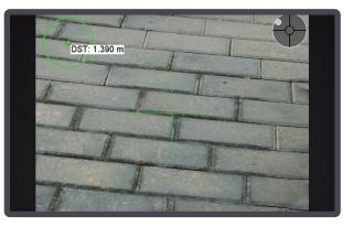
Visual Stakeout (VSO) is a convenient extension of the regular stakeout procedure. VSO makes it easier to find the target point in the field displaying the point on a special augmented reality screen which can be accessed during a regular stakeout process.
