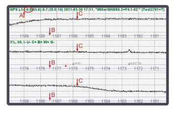
Numbers marked "A" on top left of the spectrum screens show the power of interference. The interference may be in-band or out-of band or a very wide "white noise".
