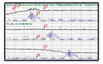
The blue line (marked "B") is the control voltage and fluctuations there shows the presence of unwanted signals with some visual quantification.
