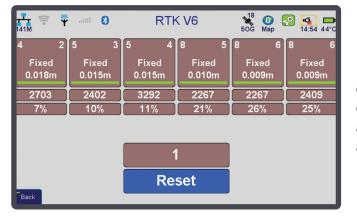
Each of our 6 parallel RTK engines employs different algorithms to calculate solutions and the weighted average of them provides robust, accurate, and fast results.
