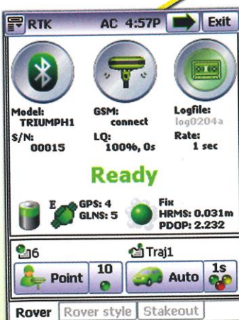
RTK (Real Time Kinematics) SURVEY AND STAKEOUT Wide set of coordinate systems including local and user defined. Ability to use global, regional and user defined (with Tracy Tools) geoids
