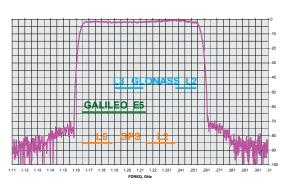
Don't worry if FCC ever authorizes any broadband wireless near GPS L1 band. We already have proven technology to protect not only against this particular one, but against all similar systems in all GNSS bands. It is implemented and fully tested option in our GNSS antennas. Our nation can have full benefits of high precision GNSS (no performance degradation at all) and full benefits of broadband wireless.
