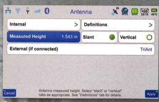
Enter antenna height and specify the type of external antenna, if an external GNSS antenna is connected.
