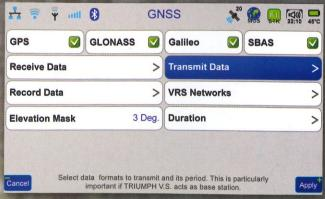
Program the receiver to act as a base station and transmit RTCM messages every second via Ethernet.
