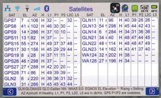
Satellites detail screen, which shows satellites names azimuth, elevation angles, health status.
