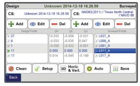
In this preliminary localization, I fixed only one point (point L011\_A). Three of the remaining four show very low residuals, however point L017\_A, with its noticeably higher vertical residual suggests this point has been displaced since it was established in 2000, or that there is an error in the observation itself - only a repeat occupation will tell.
