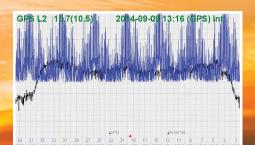
Built-in GNSS Spectrum Analyzer to detect interference in all GNSS bands.
