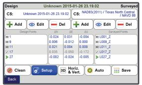
I set both the rotation and scale to zero as I do not want to redefine North nor the US Survey Foot. Now that more than one point is involved vertically, a tilted plane is calculated. Because the Stanger survey was based on Geoid96 and today's survey is based on Geoid12A, I left the tilt values intact. In this case the inclination values are so small as to be practically insignificant.
