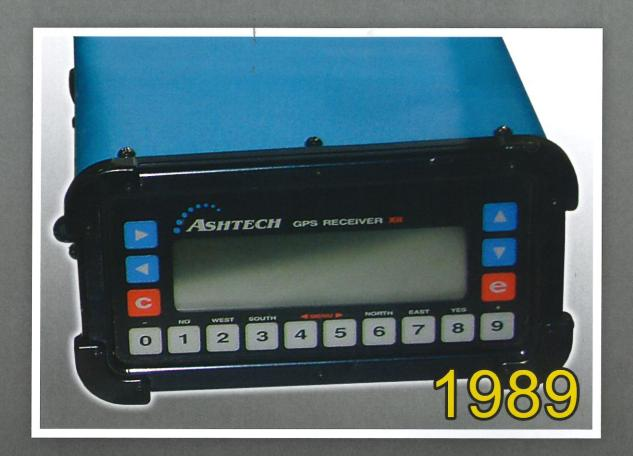
I founded Ashtech and in 1989 we introduced the first All-in-One, All-in-View 12-channel Ashtech L-12 GPS receiver, followed by Ashtech Z-12. These were the first truly portable geodetic receivers. We were also the first to integrate GPS and GLONASS satellites.
