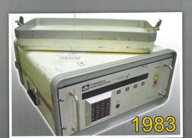
In 1983 I co-pioneered high precision GPS at Trimble, introducing the four-channel Trimble 4000-S geodetic receiver. I single-handedly wrote its complete software. It was the first commercial GPS geodetic receiver and it changed the geodetic survey industry.
