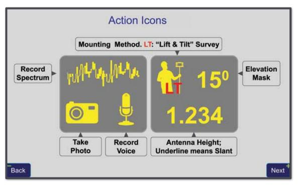
• In Lift & Tilt mode ("LT") you only need to lift the unit to near vertical on top of the survey point to start survey and then to tilt it to end the survey.
