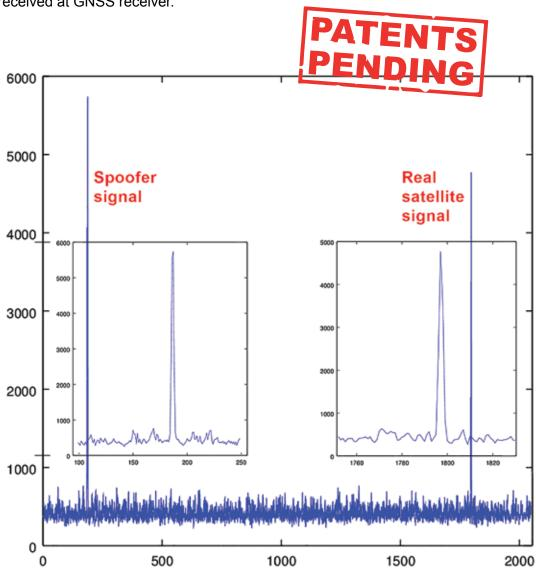
Figure below shows an example of a spoofer signal and a real satellite signal received at GNSS receiver.
