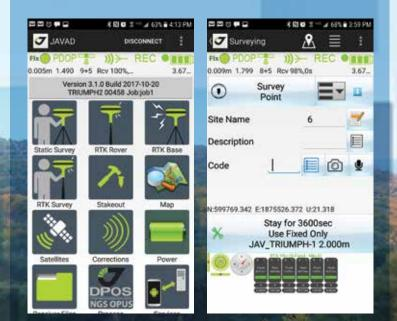
Javad Mobile Tools (JMT) is an RTK & static control software app which allows you to connect JAVAD GNSS receivers to Android or iOS devices. JMT includes a full set of RTK and static survey routines including, data collection (RTK and static), RTK stakeout, CoGo, localization and more.
