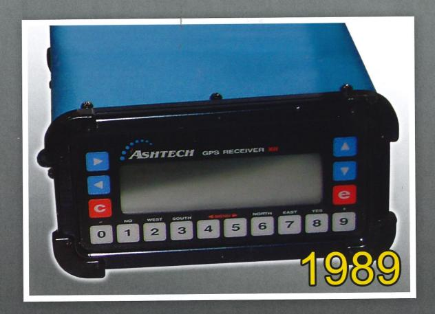
I founded Ashtech and in 1989 we introduced the first All-in-One, All-in-View 12-channel Ashtech L-12 GPS receiver, followed by Ashtech Z-12. These were the first truly portable geodetic receivers. We were also the first to integrate GPS and GLONASS satellites.
