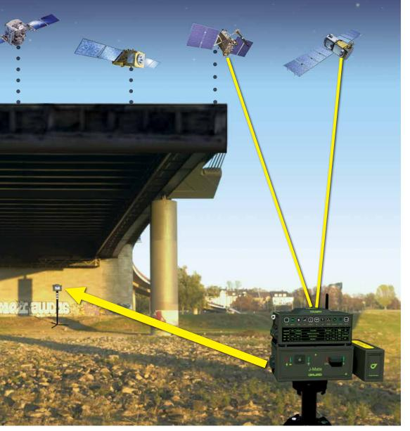
J-Mate is a bridge between RTK and areas that GNSS signal is not available.
