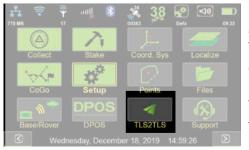
You can send and receive text messages and files from and to other TRIUMPH-LS units. In the Main screen click TLS2TLS and then in the "Compose" screen, click and enter names and serial numbers of the TRIUMPH-LS units that you want to communicate with. You
