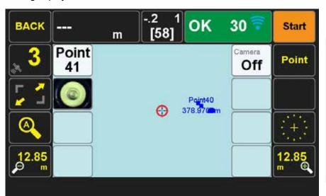
Shown here is just one example of the visual presentation of information given the surveyor. It includes being able to see at a glance the image of the rod bubble beneath the instrument's second camera and the textual display of Triumph-LS's internal pitch and roll values.
