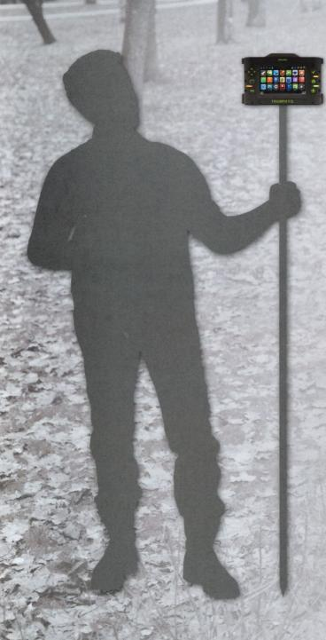
Then, go to the survey mark, lift TRIUMPH-VS to near vertical (better than 5 degrees). Survey will start automatically and sensors continuously compensate for leveling offsets. Audio tones keep you informed of the survey progress. You can use a headset if you are in noisy area. You can also take notes by talking to TRIUMPH-VS.
