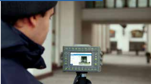
Quickly measure angles with TRIUMPH-LS internal camera by pixel processing to about 10 angular minutes.
