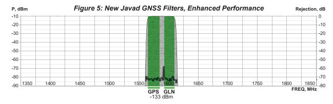
The performance difference between the old filter of **Figure 4** and new filter of **Figure 5** is enormous. The red section in **Figure 6**, below, illustrates the extra noise and undesirable signals that our old filter was allowing to pass from the antenna into the receiver. All of that extra noise degrades the performance of GNSS receivers.
