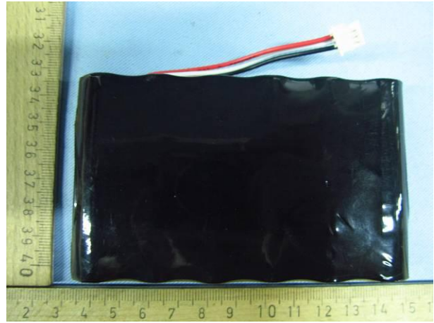
Battery/电池 (24-630101-01 7,2V 8,85Ah 63,72Wh)
