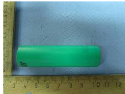
电芯/cell(NCR-18650A 3,6V 2950mAh 10,6Wh)
