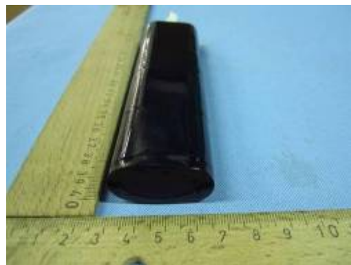
电芯/cell(NCR-18650A 3,6V 2950mAh 10,6Wh)
