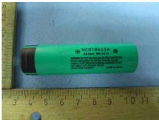
电芯/cell(NCR-18650A 3,6V 2950mAh 10,6Wh)
