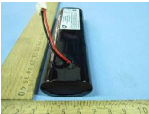
电芯/cell(NCR-18650A 3,6V 2950mAh 10,6Wh)
