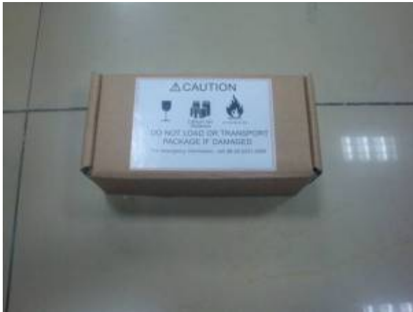
跌落测试后/after drop test
